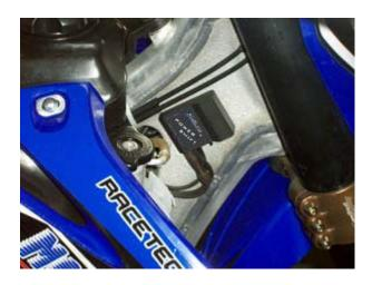
The small electronic control unit enables the user to set up the trip threshold and the cut off time.
